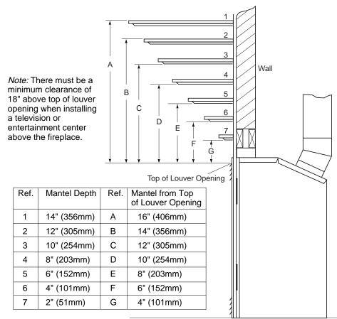
Figure 7 - Clearances for Combustible Mantels
